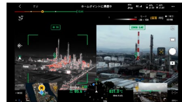
Left: Result of temperature detection by a drone Right: Aerial image captured by a drone
